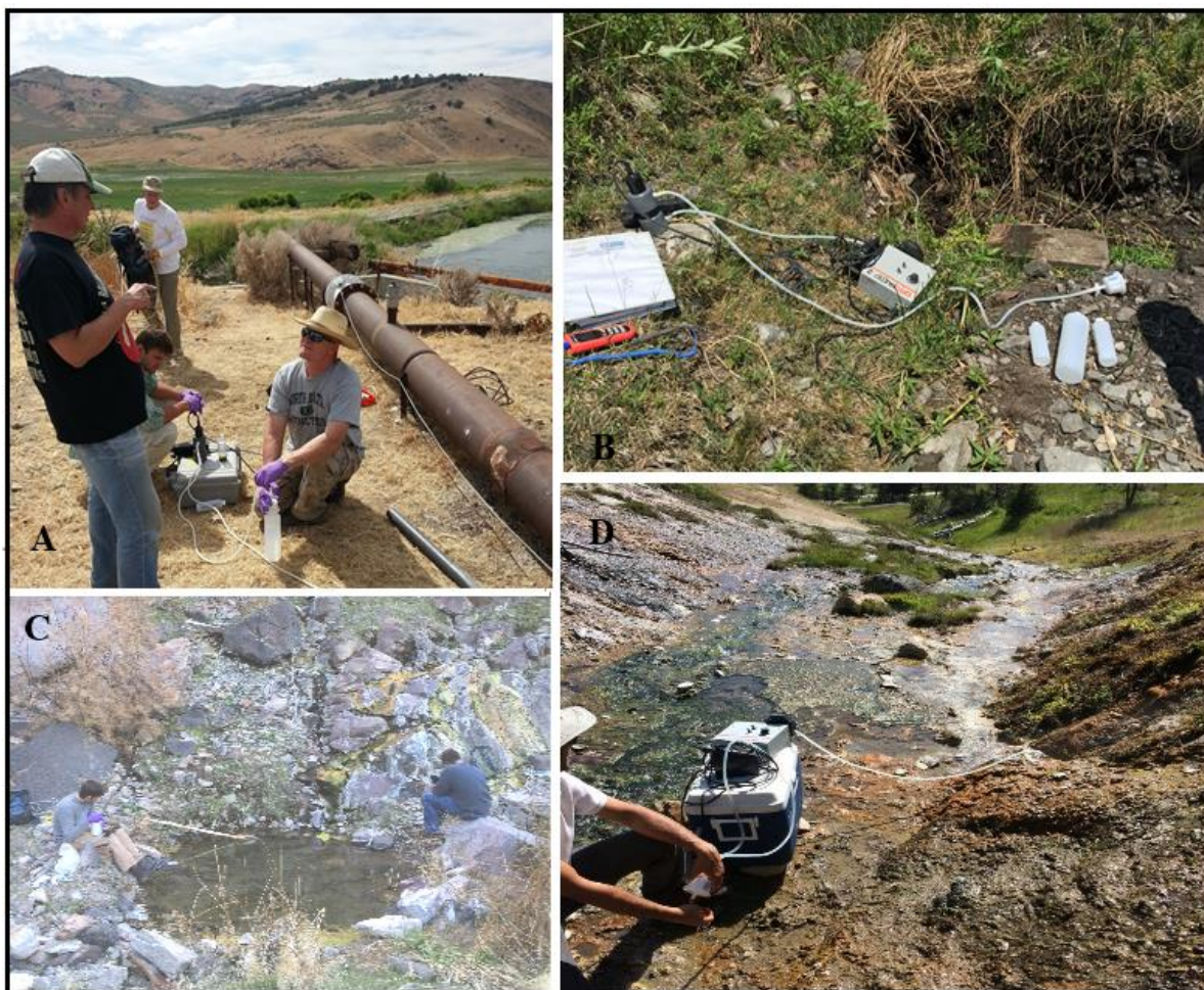
Figure A1. (A) Sample team comprised of U of I graduate student Cody Cannon (mid left), INL scientist Travis McLing (mid right), Dr. Mark Conrad (foreground) of the LBNL, and Dr. Pat Dobson (background) of the LBNL. (B) Sample equipment set up showing the peristaltic pump and tubing, 0.45 \mu m filter, YSI ® Professional Plus Multimeter and Flow-Through Cell, and three sample bottles. (C) Sampling of Driscoll Spring near Twin Falls, ID. (D) Utilization of a coiled cooling system prior to sampling collection at Worswick Hot Springs, ID.
